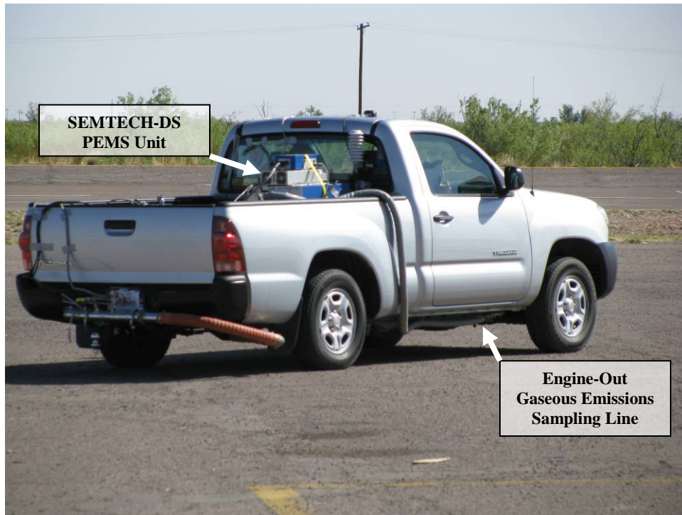
Figure 4. Emissions Measurement Unit Installed on the Test Vehicle.
