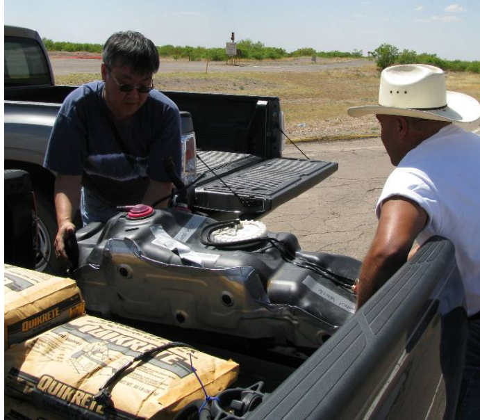
Figure 1. Toyota Tacoma Original Fuel Tank Used in the Gravimetric Fuel Consumption Measurement.
