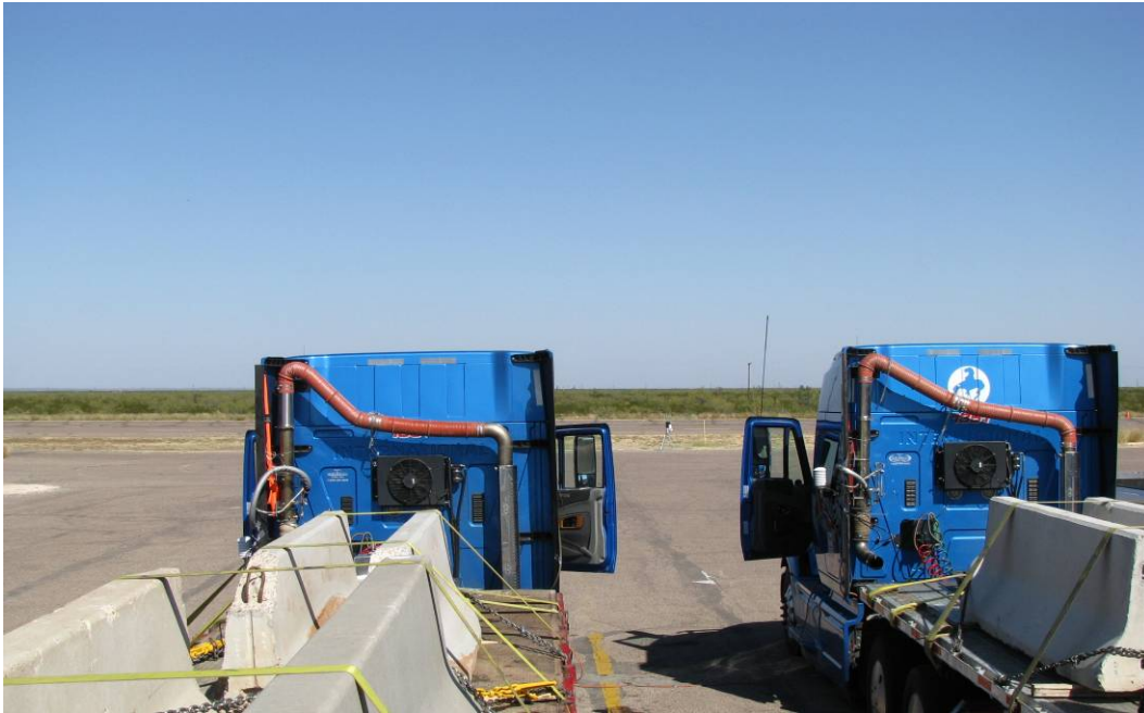
Figure 3. SEMTECH Electronic Flowmeter Installed on Tested Vehicles.
