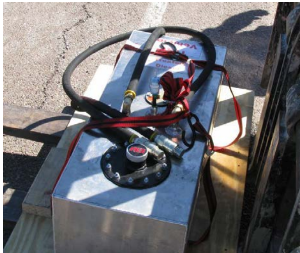
Figure 1. Auxiliary Tank Used in the Gravimetric Fuel Consumption Measurement.
